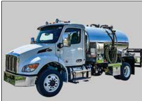
2,000-GALLON ALUMINUM, NVE 304 PUMP, 2024 PETERBILT 536, 2" INTAKE W/ HOSE, WASH DOWN HOSE. STOCK #13154. CALL FOR PRICE
