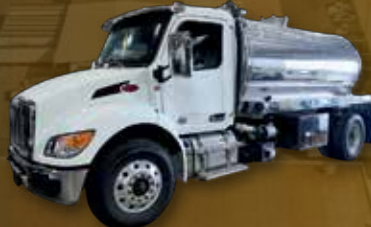
2025 PETERBILT 537 , CUMMINS ISL 9 300 HP, ALLISON 3000 RDS AUTO. TRANSMISSION, 2500 ALUMINUM TANK, JUROP RV 360 - 360 CFM, 36" ALUM. TOOLBOX, 33K GVWR. PRICE $182K + FET | STOCK #55
