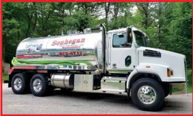
⬆️ Souhegan Septic Tank Service's 2023 Mack built out by Imperial Industries with a 4,250-gallon aluminum tank and National Vacuum Equipment 4310 blower.
