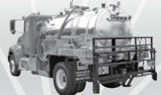
Truck mounted portable toilet services units
