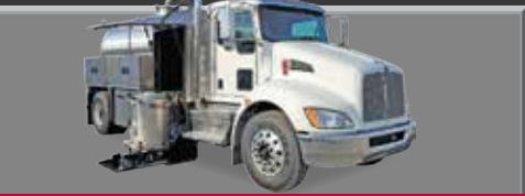
USED T370 KENWORTH GREASE TRUCK 300 HP, ALLISON AUTO, 33,000 (G.V.W.R.), 1800 GALLON STAINLESS STEEL (TI) TANK, NVE 607 PROMAX PACKAGE, HEAT COLLARS (HEAT THROUGH TANK), HEATED CABINET FOR PROVAC UNIT W/ HYDRAULIC LIFT, HANNAY HOSE REEL W/ 100' 2" HOSE IN HEATED CABINET.
