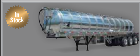
7000 - 9000 GAL. ALUMINUM TRI-AXLE TRAILERS AIR RIDE SUSPENSION (TRI-AXLE), PUMP PLATFORM, BRIGHT FINISH, LED LIGHTS, BETTS VALVES.
