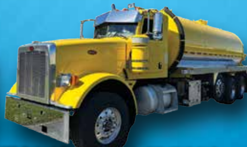
2012 Peterbilt 367 - Cummins ISX15 485 HP, 8LL Trans., 5,000 Gallon Steel Tank, NVE 4310 BLOWER Package(940 CFM), Flotation Tires, 20K Front Axle, 36" Alum.Toolbox, Betts Lights, LOW MILES - Call for Price -
