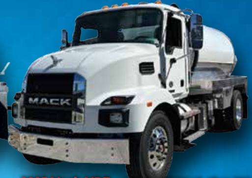
2025 Mack MD7 - Cummins ISB 260 HP, Allison 2500 Auto. Trans., 2,500 Gallon Steel Tank, NVE 607 Pro Max Package (380 CFM), 24" Alum. Toolbox, Chrome Package, 33k GVW - $138,000 -
