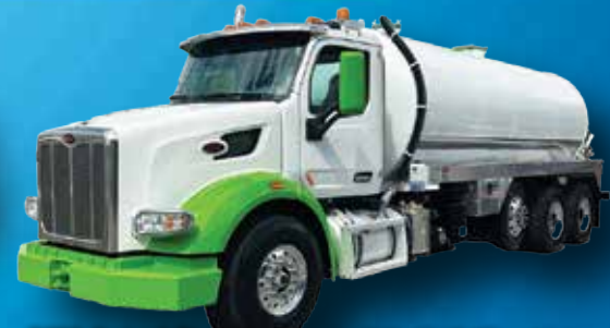
2018 Peterbilt 365 - Cummins ISX15 450 HP, 13Speed Auto Trans., 5,000 Gallon Steel Tank, NVE 877 PRO MAX (538 CFM), Aluminum Wheels, Heavy Duty Front Bumper, Heavy Duty Jetter, 48" Alum.Toolbox, Jeter Betts Lights, LOW MILES - Call for Price -
